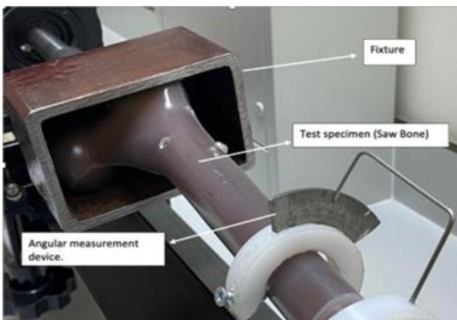
The torsion test was applied to create an angular displacement of 10 degrees and the maximum load required to create the rotational displacement was noted. No load was exerted axially along the femur during torsion testing, thus avoiding frictional resistance at the fracture site. The load/Torque applied was measured in Newton meters (Nm) using digital torque measuring machine (TeCQuipment E -101 Digital Measuring System)
