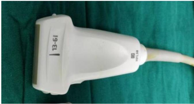
Figure 8: Ultrasound machine with 13-6MHz probe (Sonosite S-Nerve)
