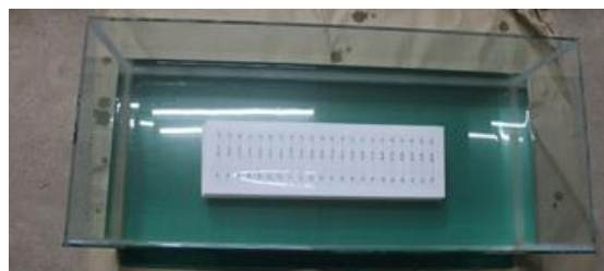
Figure 3: Custom-made acrylic plates immersed in artificial saliva
