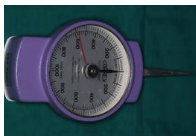
Figure 4: Force measuring instrument (Correx gauge)
