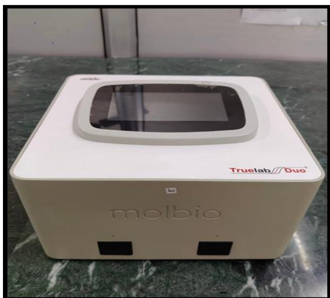
Figure 1: Truelab Duo real-time PCR analyzer used for HLA-B27 detection
